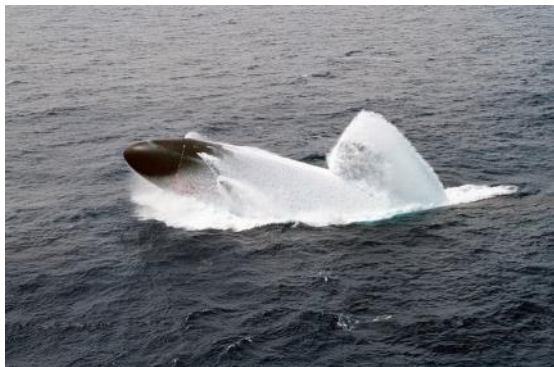
USS Columbus (SSN 762) performs an emergency blow off the coast of Oahu, Hawaii, during a training drill, June 1998.
